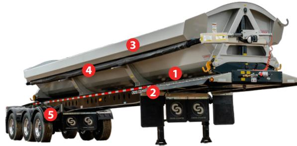
1. Hardox® 450 premium wear plate material provides exceptional durability, available in 3/16" & 1/4" thicknesses
