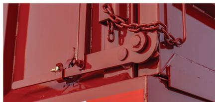
Ground controls for unlocking tailgate
