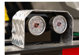
Two load scale gauge boxes located at front, protected by aluminum guard
